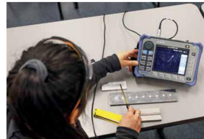
Ybarra gains skill in ultrasonic testing in Penn College's nondestructive testing lab, inside its 55,000-square-foot Lycoming Engines Metal Trades Center. Today, Ybarra examines weld quality on Harley-Davidson parts.
