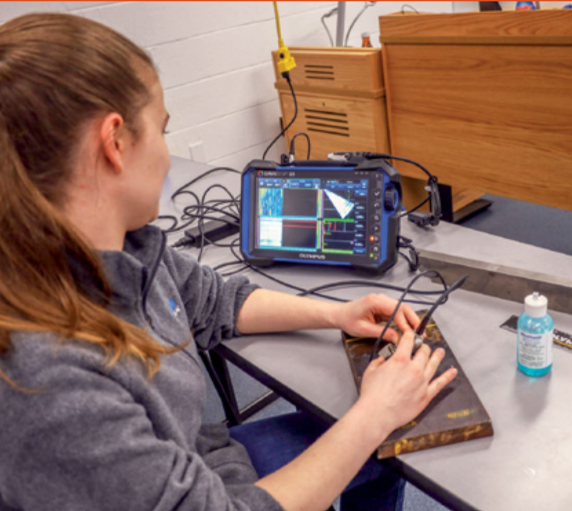
A student in Penn College’s nondestructive testing major uses ultrasound technology to detect flaws in a weld.
