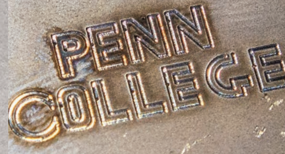
At top: A newly joined pair of pipes are seated in the college’s new 60kV electron beam welder. Instead of using a filler material, the heat from high-speed electrons melts and joins the materials, providing for a very thin welding bead. At bottom: A sample of the welder’s etching work. The actual size is about an inch wide.
